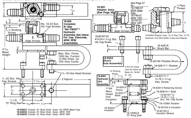
We recommend using a Fire Resistant Hydraulic Fluid compatible with BUNA "N" such as HOUGHTO-SAFE #620, 1120 or equivalent.
